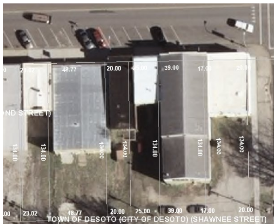
Figure 16 Commercial Setbacks. Commercial buildings typically do not observe side setbacks and often have shared side walls. The rear of the lot can then be used for storage, parking and deliveries.
