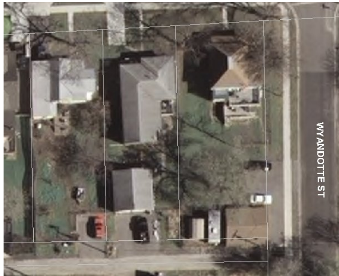
Figure 15. Residential Setbacks. The center home above makes good use of the lot by setting the home off to one side, placing the garage in the rear of the home—accessible from the alley. The home and the garage are each 20' from the front and rear property lines respectively. The 15' on the west side of the house would be sufficient for a driveway if the alley was not available. The lot is 50' x 150'.
